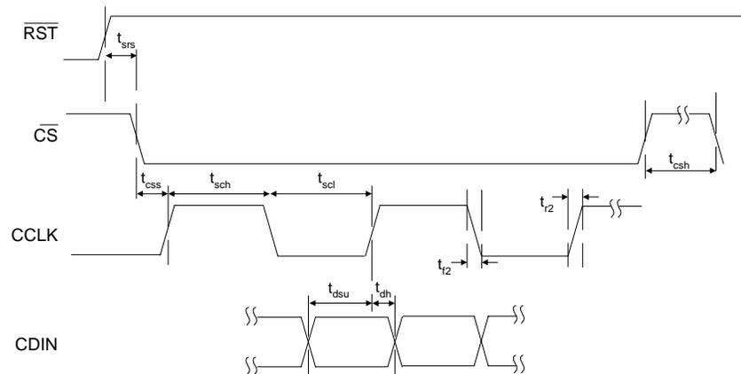
**Figure 7. Control Port Timing - SPI Format**
