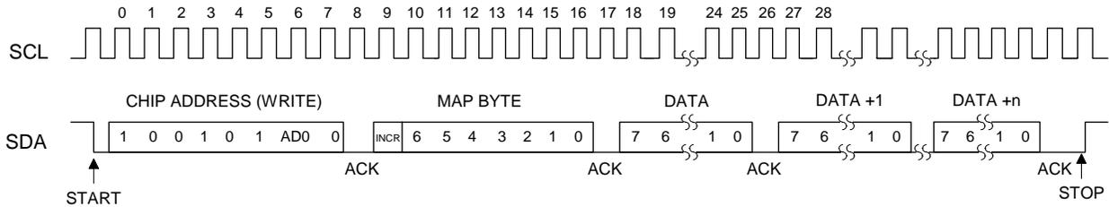
**Figure 24. Control Port Timing, I<sup>2</sup>C Write**
