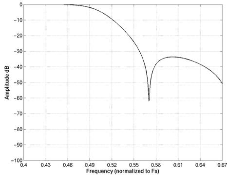
**Figure 36. ADC Transition Band**
