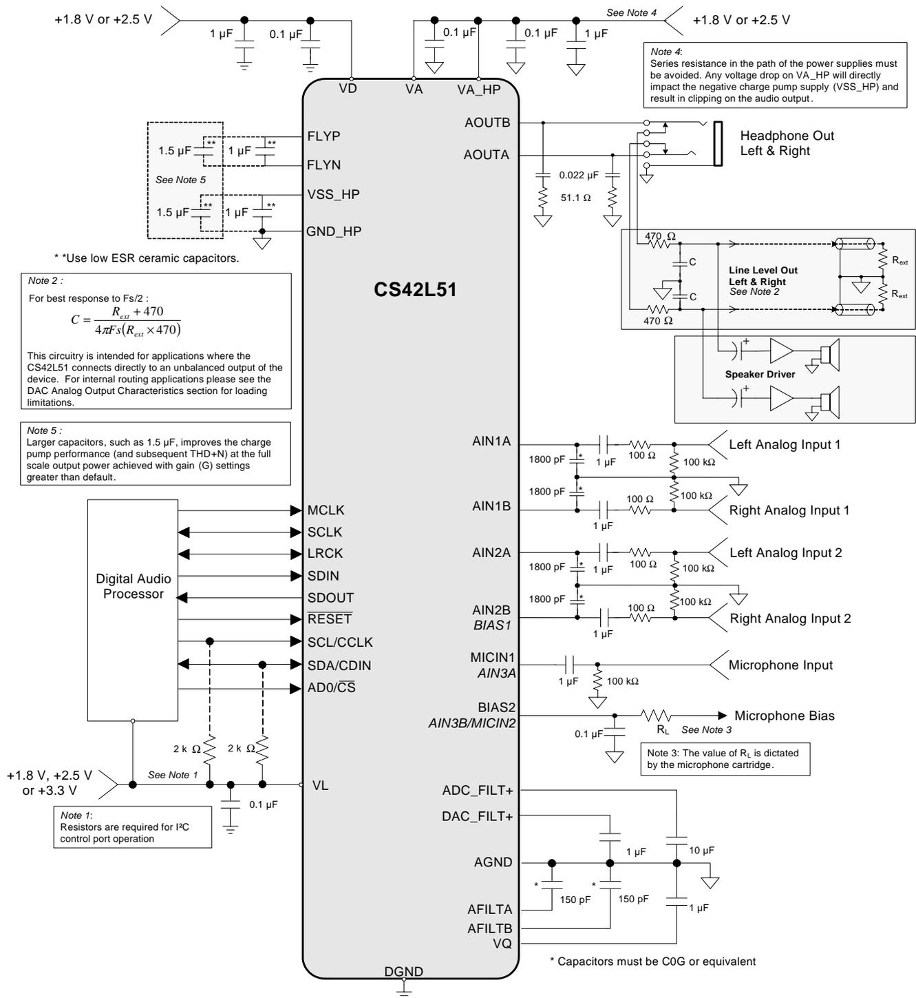
Figure 1. Typical Connection Diagram (Software Mode)
