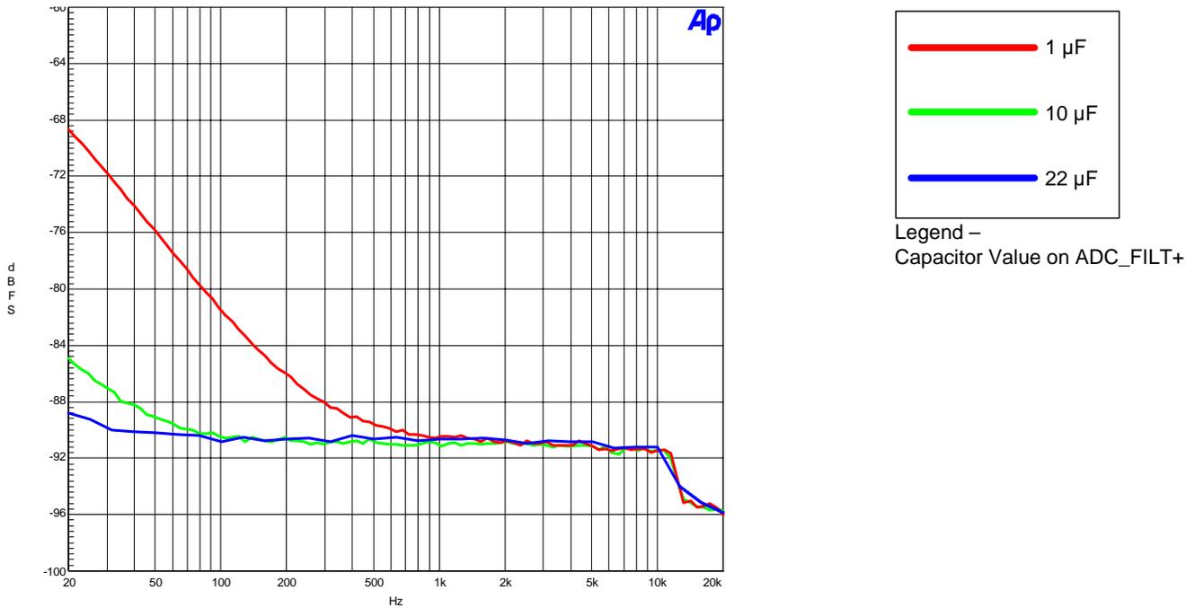
**Figure 33. ADC THD+N vs. Frequency w/Capacitor Effects**
