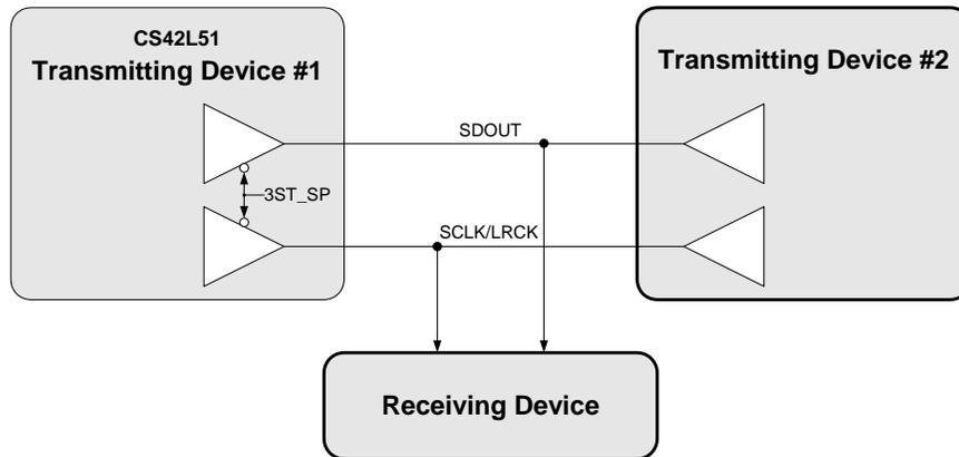
Figure 18. Tri-State Serial Port
