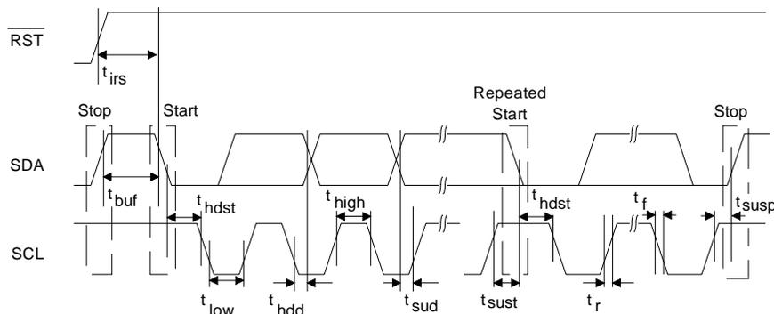
**Figure 6. Control Port Timing - I<sup>2</sup>C**
