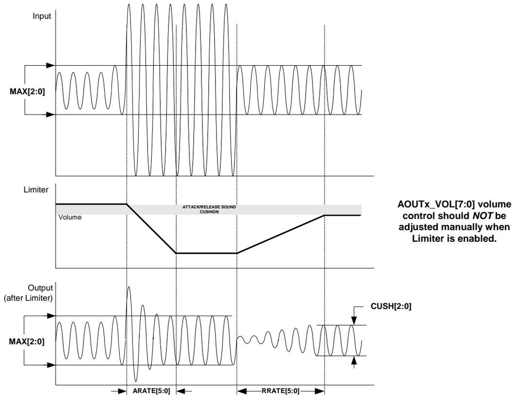
**Figure 16. Peak Detect & Limiter**
