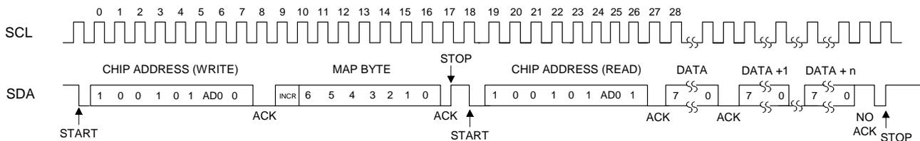
**Figure 25. Control Port Timing, I<sup>2</sup>C Read**
