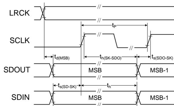
**Figure 5. Serial Audio Interface Master Mode Timing**
