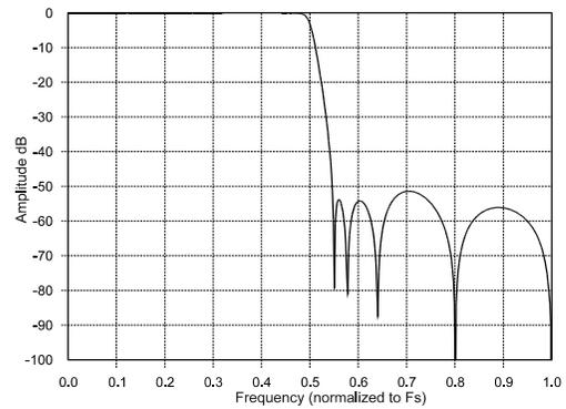
**Figure 39. DAC Stopband**
