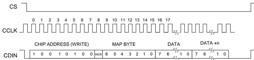
**Figure 23. Control Port Timing in SPI Mode**
