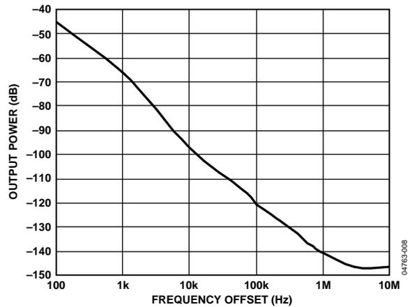
Figure 8. Open-Loop VCO Phase Noise, L1, L2 = 110 nH
