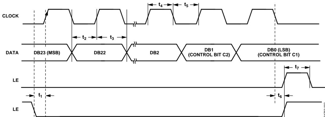
Figure 2. Timing Diagram
