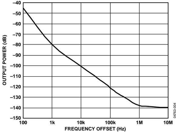
Figure 4. Open-Loop VCO Phase Noise, L1, L2 = 560 nH
