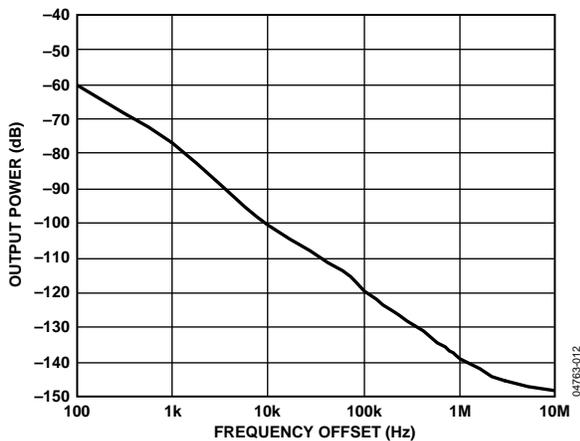
Figure 12. Open-Loop VCO Phase Noise, L1, L2 = 18 nH
