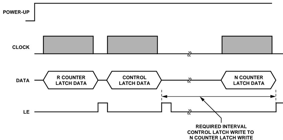
Figure 21. ADF4360-8 Power-Up Timing
