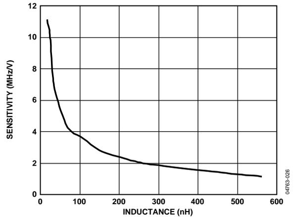
Figure 23. Tuning Sensitivity (in MHz/V) vs. Inductance (nH)
