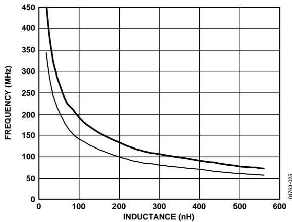
Figure 22. Output Center Frequency vs. External Inductor Value
