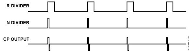
Figure 17. PFD Simplified Schematic and Timing (In Lock)
