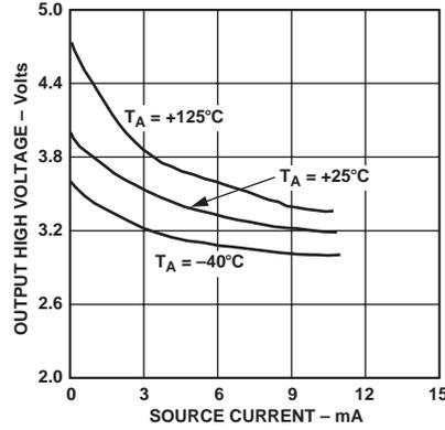
Figure 11. Output High Voltage,  $V_{OH}$  vs. Source Current
