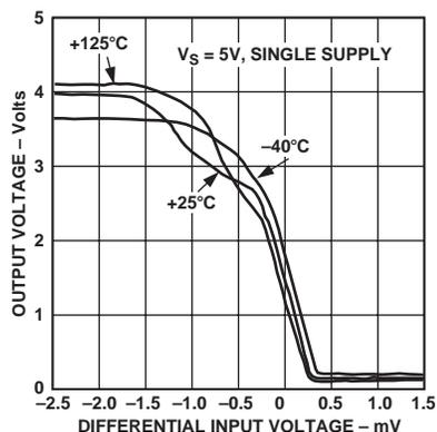
Figure 1. Output Voltage vs. Differential Input Voltage
